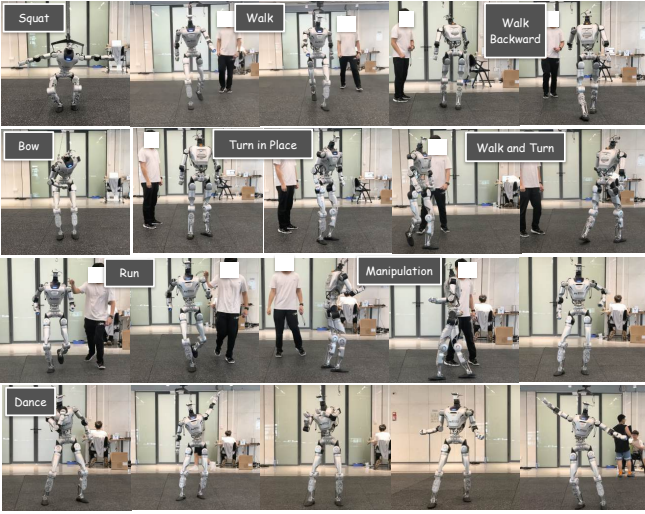
Fig. 4. Real-world deployment of the adapted Sonic-to-Oli policy after 90 GPU-hours of AMASS adaptation. Snapshots show squatting, forward and backward walking, turning, bowing, running, manipulation, and dancing.
